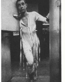
THERMAL ROOM of Aero Medical Laboratories at Wright Patterson Air Force Base tests human beings' ability to withstand heat of unfiltered sunlight in outer space. Above, wires measure Lt. Larry Colman's reactions to 190-degree heat. At plus twenty minutes he began to lose ability to solve problems, He lasted
